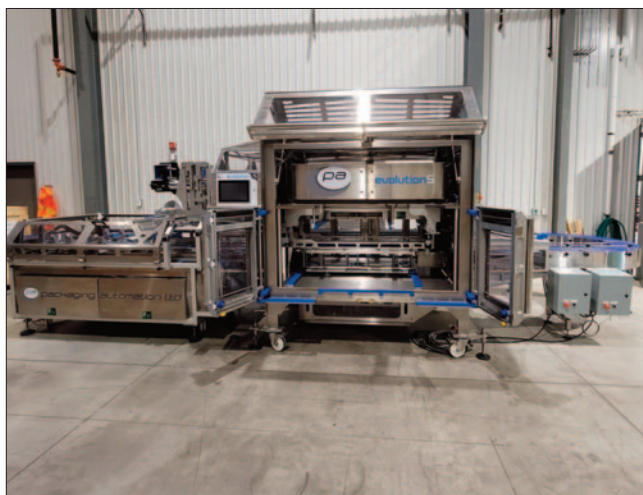
The Evolution S tray sealing system is fully automatic. Its claim to fame is the world's fastest tray sealer.
